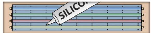
4. The holes are filled in by hand, and the cable needs to be cured again.
