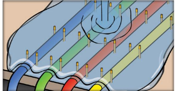
1. Wires are stretched between pins in a mold, and then liquid silicone plus additives are poured over the wires.
