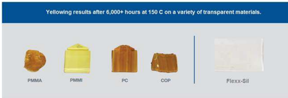
Figure 3: Yellowing in Flexx-Sil™ Material and other like Materials over 6,000 Hours.
